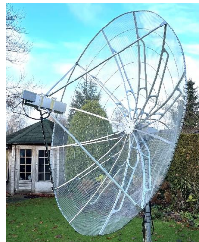
PA0TRB's new 3.5 m dish with 1296 feed
