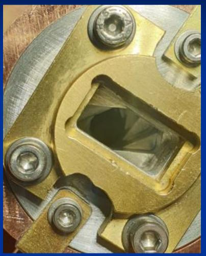
WR-75 flange (prior to solder WG)
