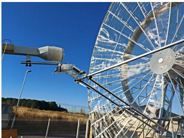
Ozařovač pro 1296MHz v offset parabole 8m OK1DFC
