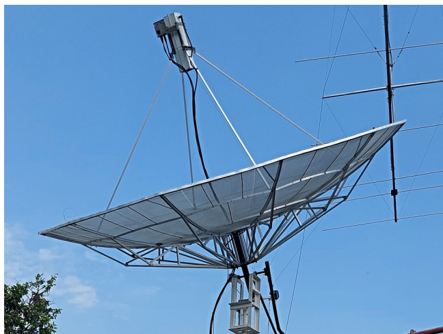
YB2MDU 4,5m parabola a 1 kW na 23cm
