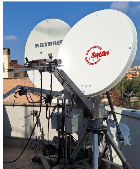
EA3HMJ's 3 cm Portable EME Demo Station
