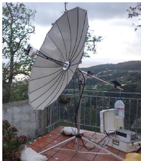
CT9/EA8DBM 1.8 m folding dish on Madeira island
