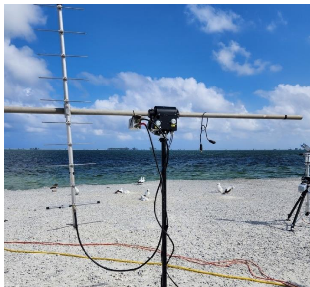
On 432 EME TX5S used an 11 el yagi with 70 W
