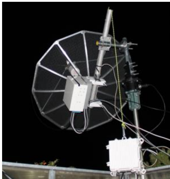
OK1TEH's 1 m dish and equipment used on 9 cm
