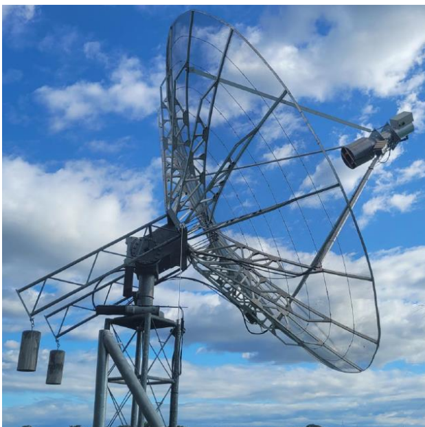
DU3T's 4.6 m dish with 9 cm feed
