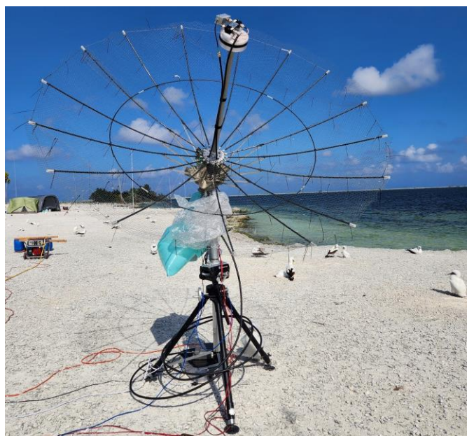
On 1296 a 2.4 m HRO dish and 400 W were used
