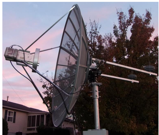
KD2XN 2.3 m Dish (f/D .375) used on 23 cm with 200 W
