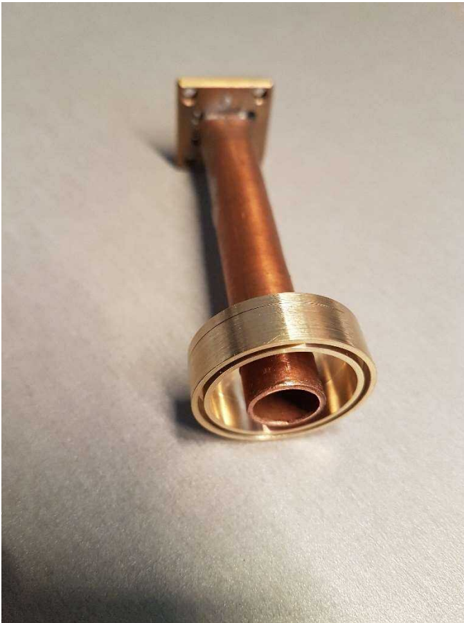
Figure 14- PA0PLY's new feed for 24 GHz
