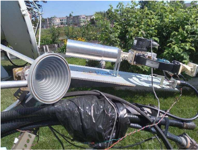
Figure 17 – VE4MA's new W2IMU feedhorn
