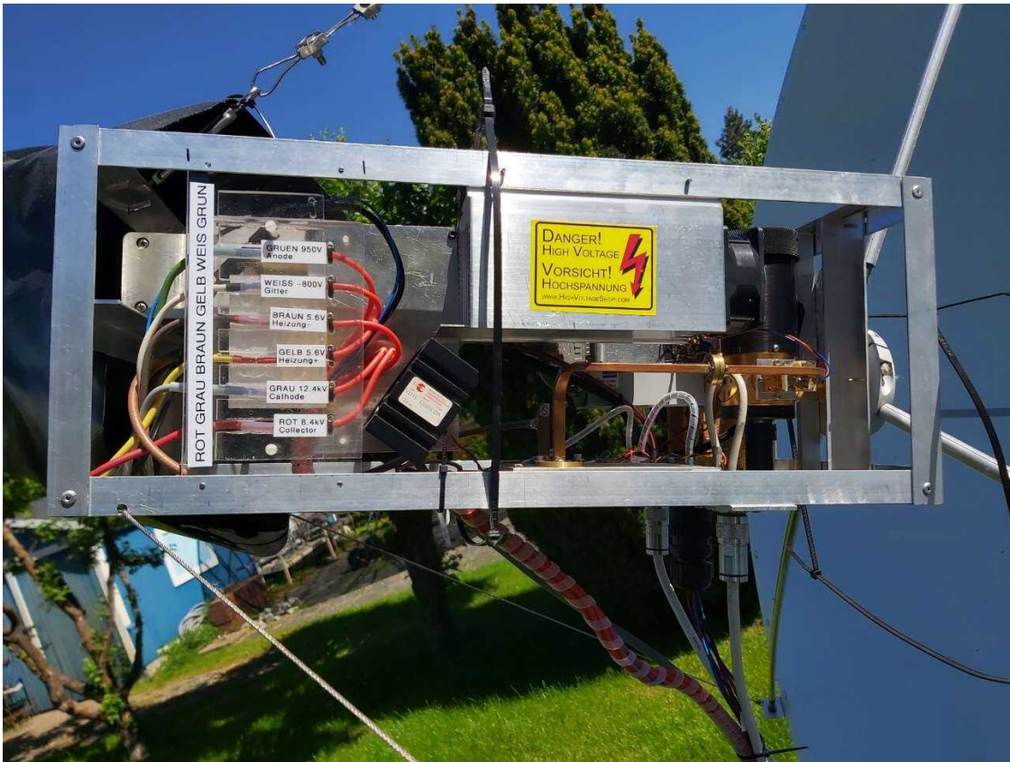
Figure 24- DL7YC 47 GHz TWT at feed
