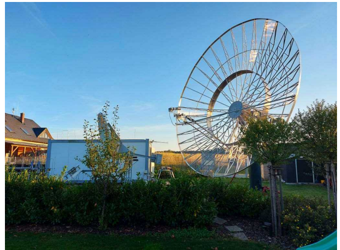
Figure 14 - OK1DFC 8m + 2.4m offset dishes for 13-3 cm
