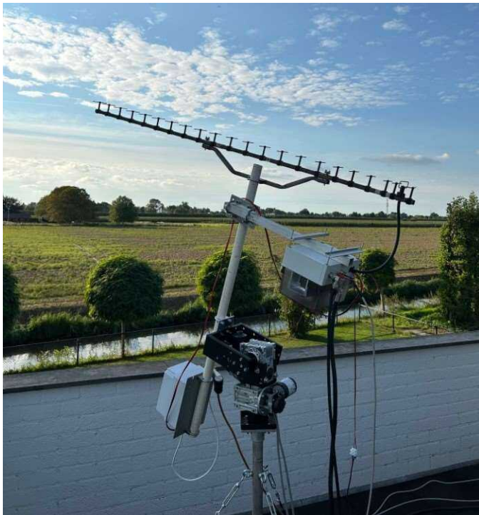
Figure 27 - PA3DZL 23el 1.75m 15.8 dBd setup
