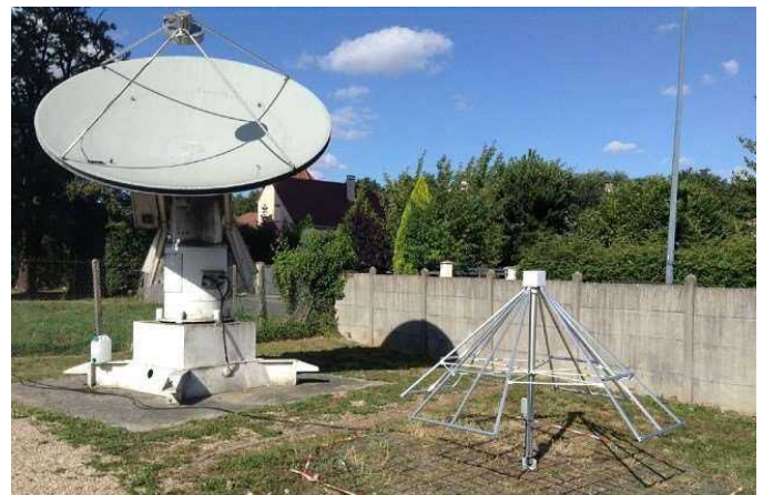
Figure 6 - F1EHN 3.3m dish + 21cm astronomy feed
