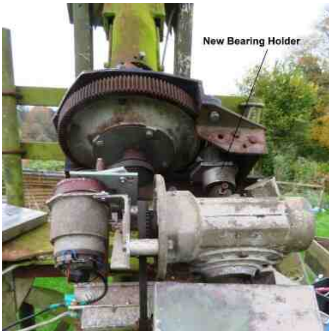
G3LTF Repaired Hour Angle Drive
