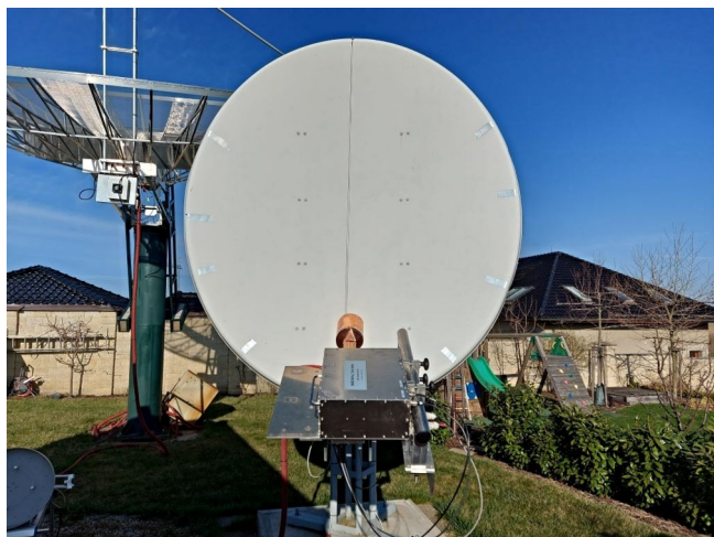
Parabola 2,4m OK1DFC s TRX pro 3,4GHz
