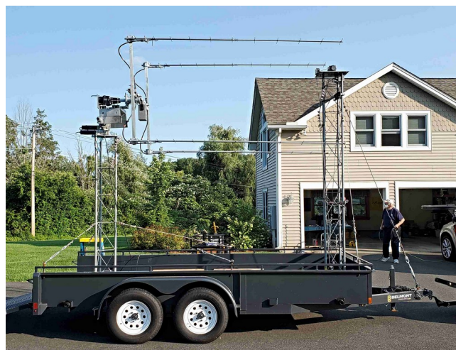
Otočný systém 4x12 el. Yagi expedice N1H
