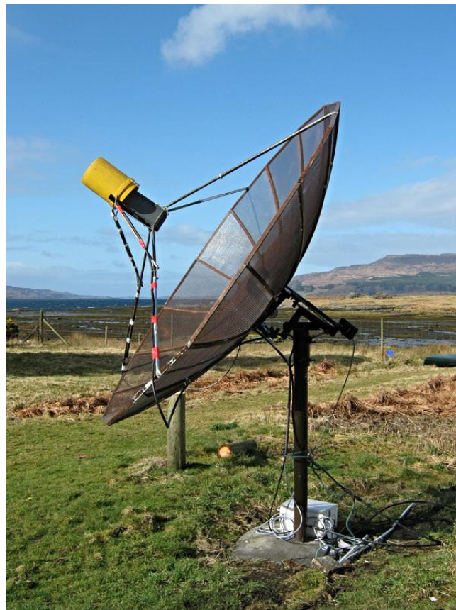
Parabola 3,2m GM4PMK pro 23cm a 9cm
